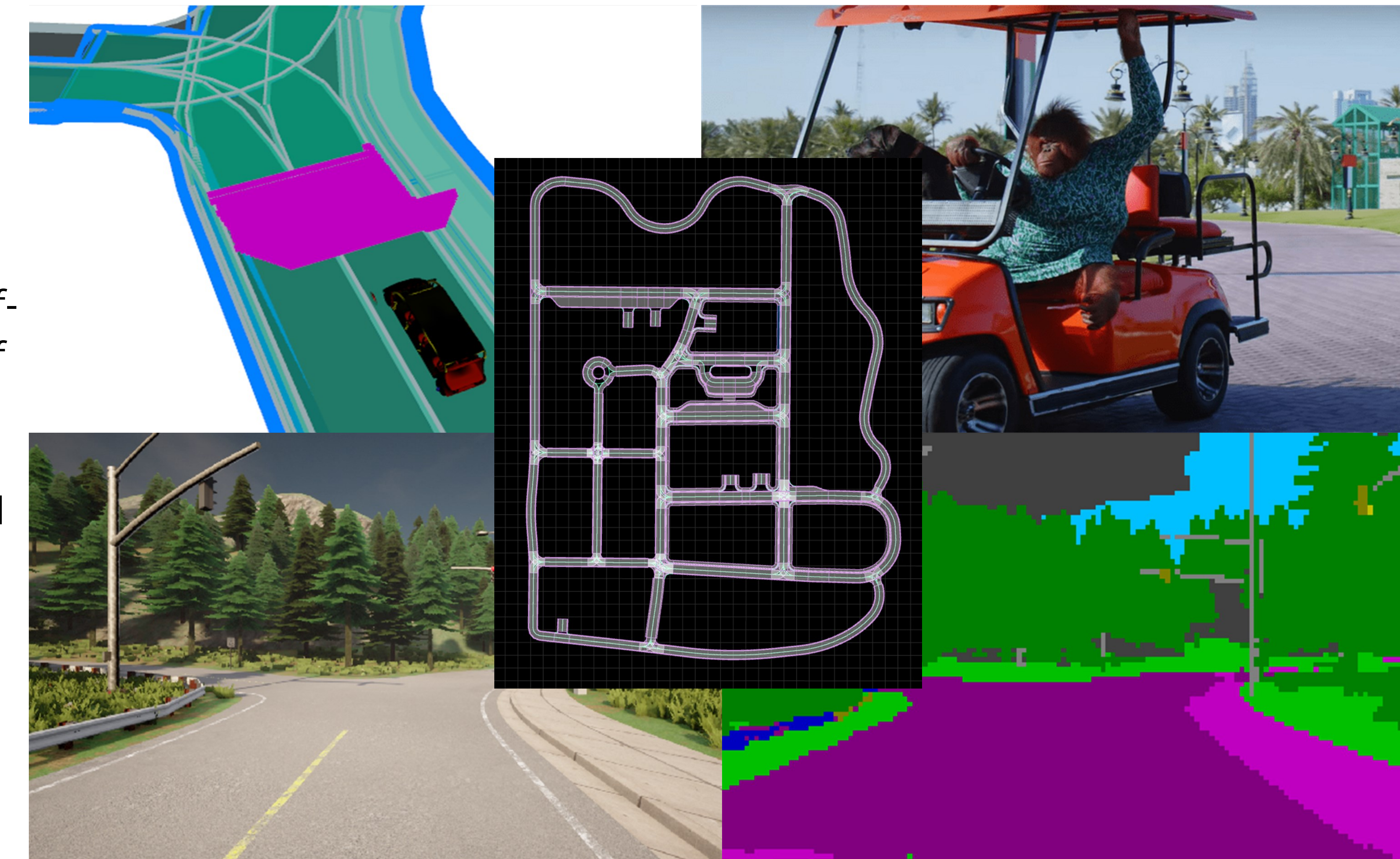
Counterclockwise and center: The car's view, including the road boundary (blue) and the identified road points (purple); an orangutan putting robots to shame; simulated camera; semantic segmentation; our HD map.
